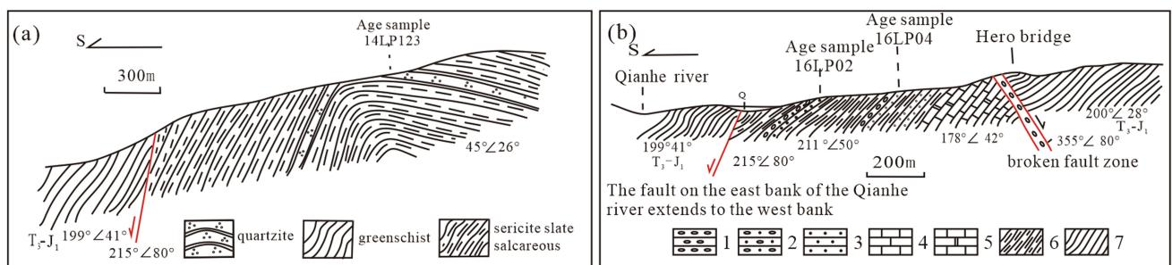
**Fig. 5** Geological section along the banks of the Qian River in the southern part of Fengjiashan Reservoir; 1. conglomerate; 2. glutenite; 3. sandstone; 4. limestone; 5. marbled limestone; 6. sericite, calcareous slate; 7. Greenschist. The age sample 14LP01 in the picture is the Youjia (2016) dating sample
