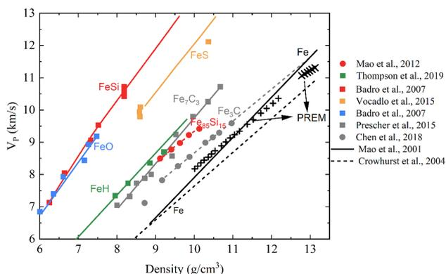
**Fig. 6** The density and  $V_p$  for Fe-rich alloys. The colored squares and circles are measured data for Fe-rich alloys, while the colored curves fit the Birch's law. The solid and dashed curves in black represent pure iron. The crosses are the outer core and inner core. The datasets are from Mao et al. (2012), Litasov and Shatskiy (2016), Chen et al. (2018), Thompson et al. (2018), and references therein
