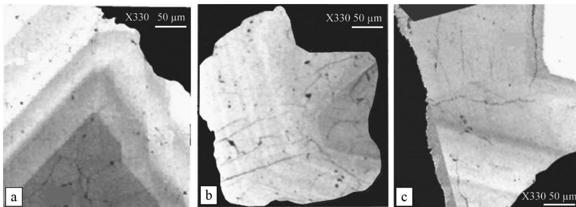
**Fig. 6** Backscattered electron images of Nb-Ta minerals from Ngoura. **a** Oscillatory zoning; **b** progressive oscillatory zoning; **c** irregular oscillatory zoning truncated in the border zone
