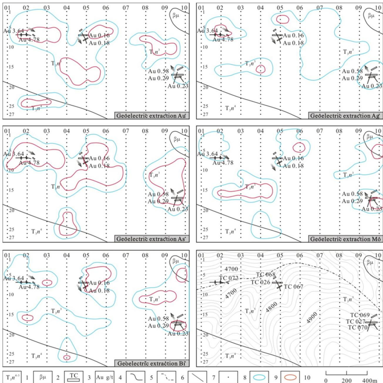
**Fig. 7** Plane maps of electrogeochemical contrast anomalies of elements in the study area. 1. Third to fourth members of the Upper Triassic Nieru Formation, 2. diabase vein, 3. exploratory trench, 4. gold grade, 5. geological boundary, 6. river, 7. vein, 8. sampling point, 9. 1.5 isoline of contrast anomalies, 10. 2.5 isoline of contrast anomalies
