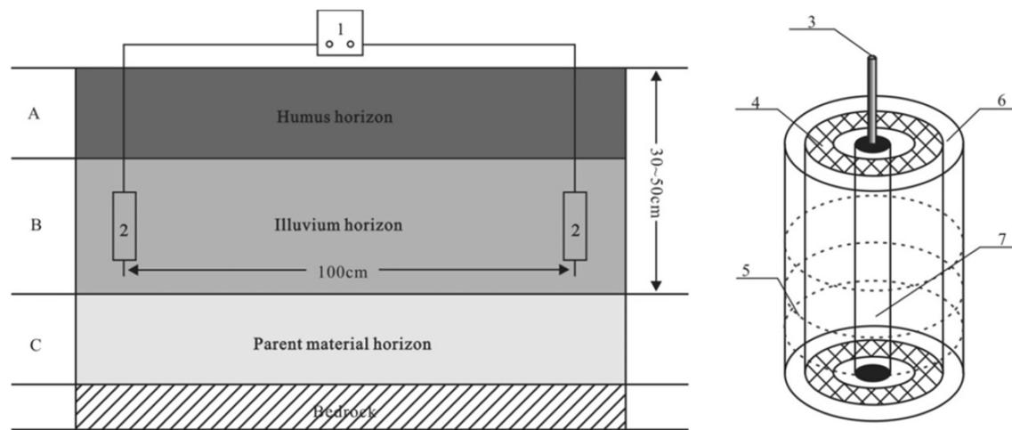
**Fig. 3** Diagrams showing sampling methods and the dipole CHIM extraction device with independent power supply. 1. Controllable power source, 2. extraction electrodes, 3. connecting wire, 4. adsorptive foamed plastic material, 5. fixed wire, 6. filter paper, 7. graphite carbon rod
