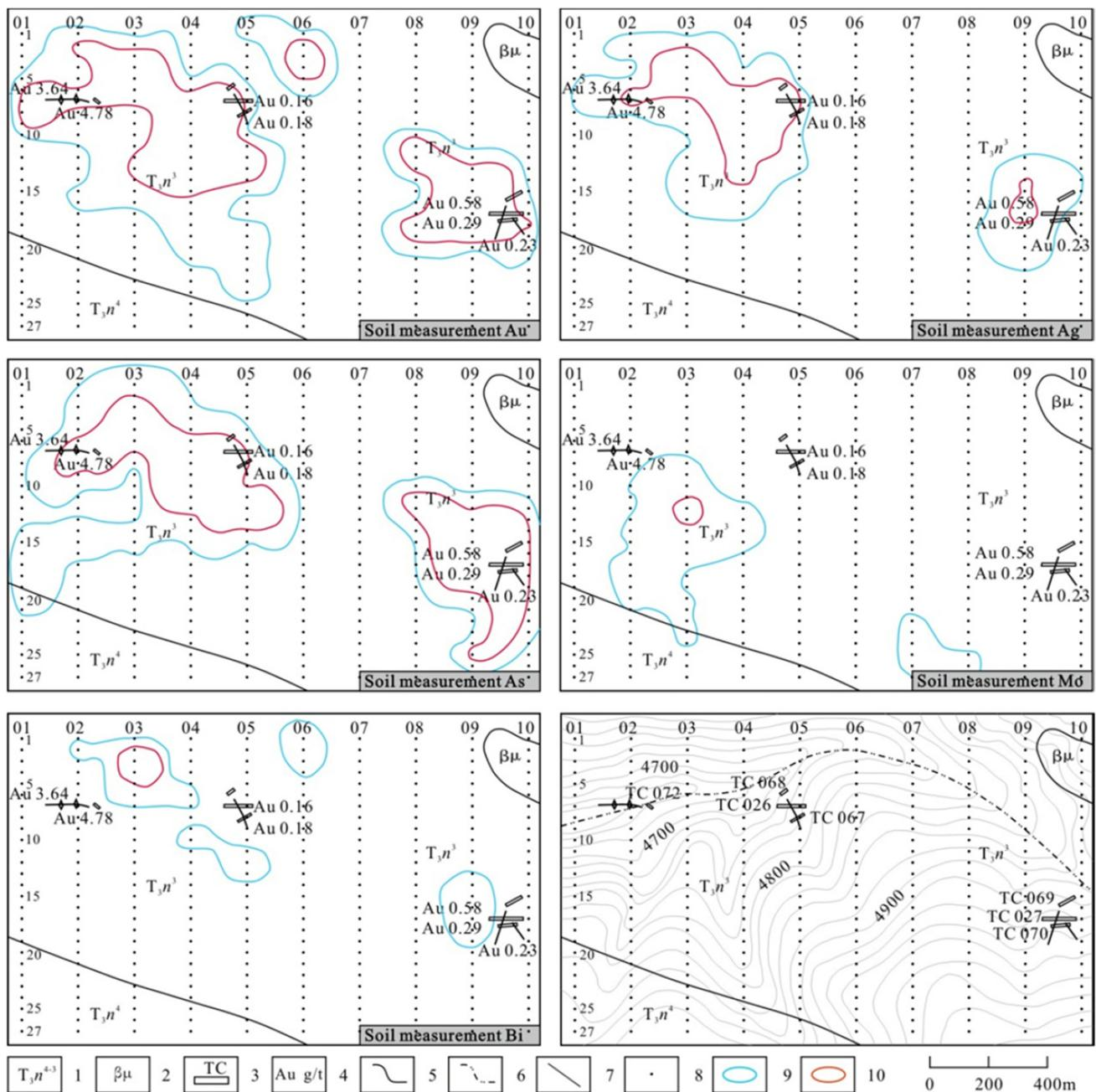
**Fig. 6** Plane maps of contrast anomalies of elements from soil measurements. 1. Third to fourth members of the Upper Triassic Nieru Formation, 2. diabase vein, 3. exploratory trench, 4. gold grade, 5. geological boundary, 6. river, 7. vein, 8. sampling point, 9. 1.5 isoline of contrast anomalies, 10. 2.5 isoline of contrast anomalies
