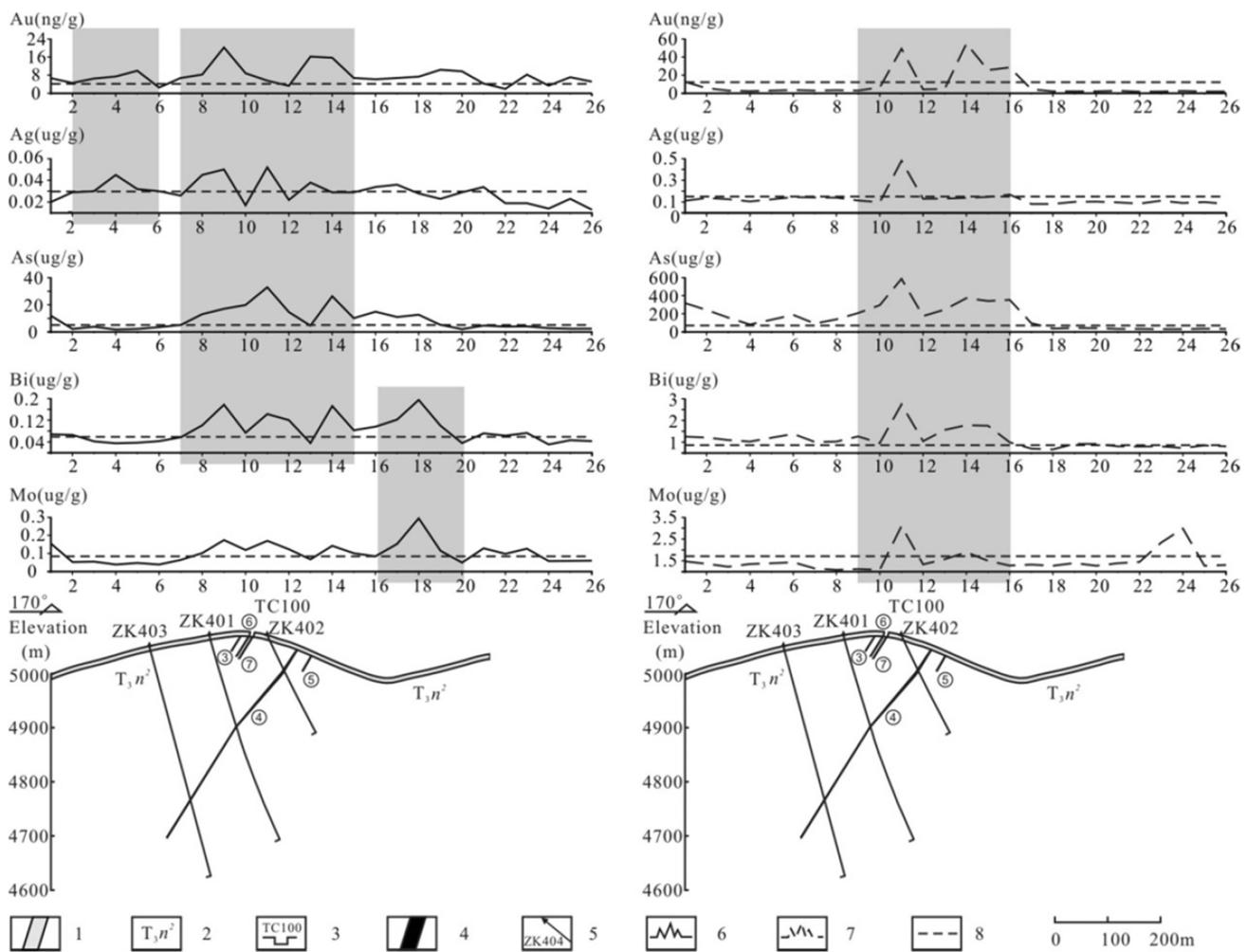
**Fig. 4** Comparison of sections derived from measurements of electrogeochemical and soil samples. 1. Quaternary, 2. second member of the Nieru Formation of the Upper Triassic, 3. veins, 4. exploratory trench and serial number, 5. perforation and serial number, 6. electrogeochemical anomalies, 7. soil measurement anomalies, 8. background value line
