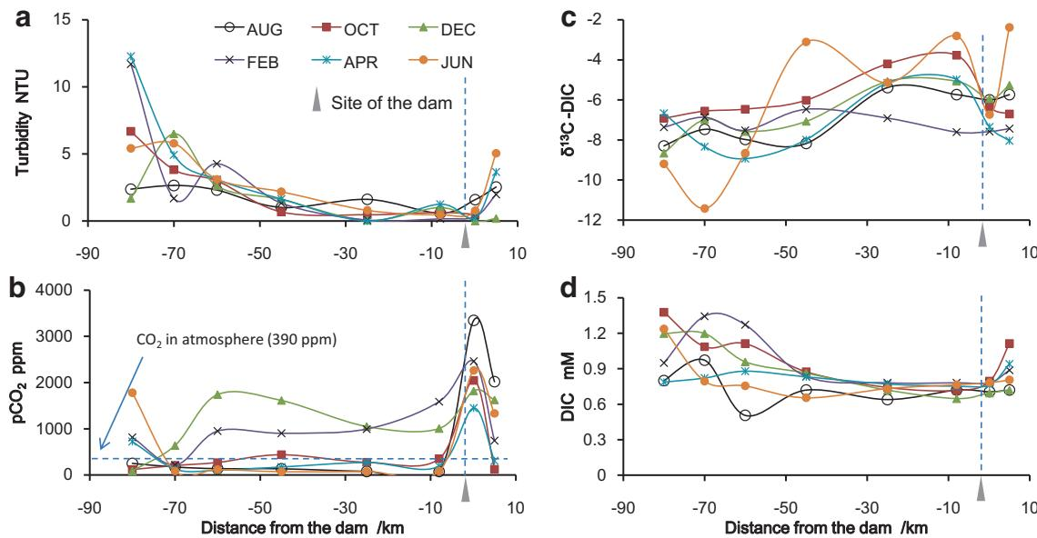
**Fig. 2** Turbidity,  $p\text{CO}_2$ , DIC concentration and its isotopic compositions in surface water along the Xinanjiang Reservoir
