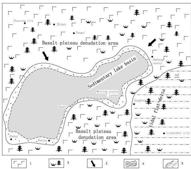
**Fig. 5** Paleogeography sketch of iron-bearing rock system. 1. Basalt plateau denudation area, 2. Cathaysia flora, 3. Transportation direction of material sources, 4. Lake basin and margin, 5. Tidal flat to delta
