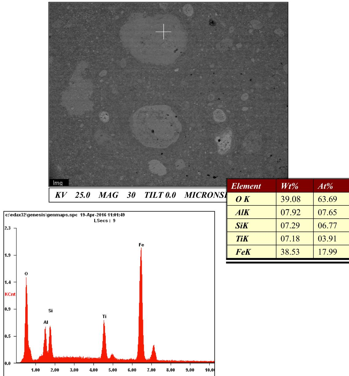
**Fig. 3** Energy spectrum analysis of scanner electron microscope (MBT2-7B-1) for Xianglushan deposit, Weining (after School of Natural Resource and Environmental Engineering 2016)
