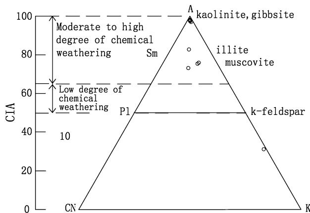
**Fig. 6** A-CN-K Ternary diagram [ $A = n(\text{Al}_2\text{O}_3)$ ,  $K = n(\text{K}_2\text{O})$ ,  $\text{CN} = n(\text{CaO}^* + \text{Na}_2\text{O})$ ] (modified after Guo and Su 2014)
