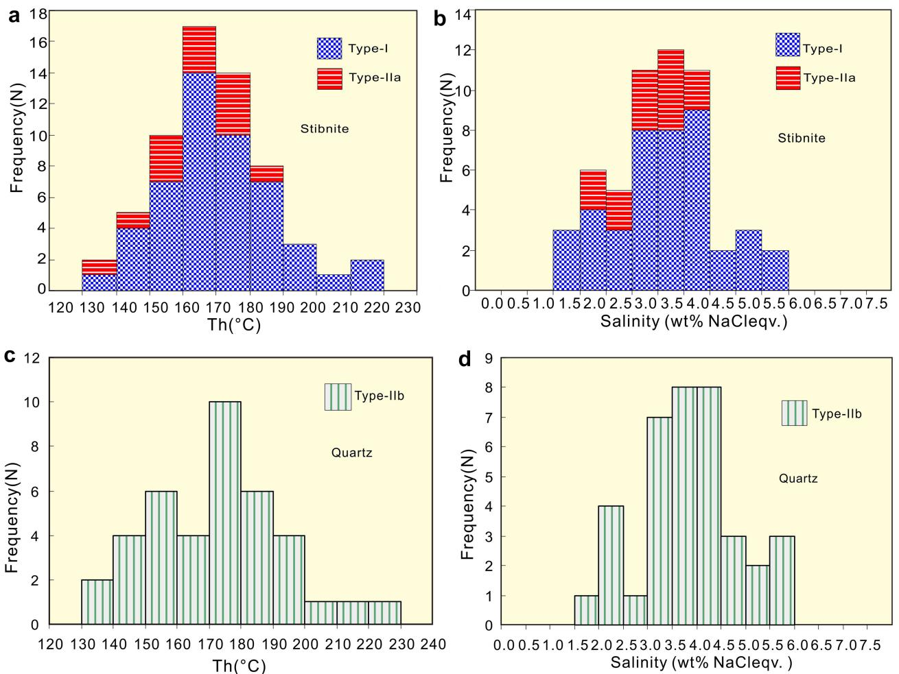
**Fig. 7** Histograms of salinities and homogenization temperatures of fluid inclusions in stibnite (**a**, **b**), and coexisting quartz (**c**, **d**), collected from the Leishan-Rongjiang antimony ore field
