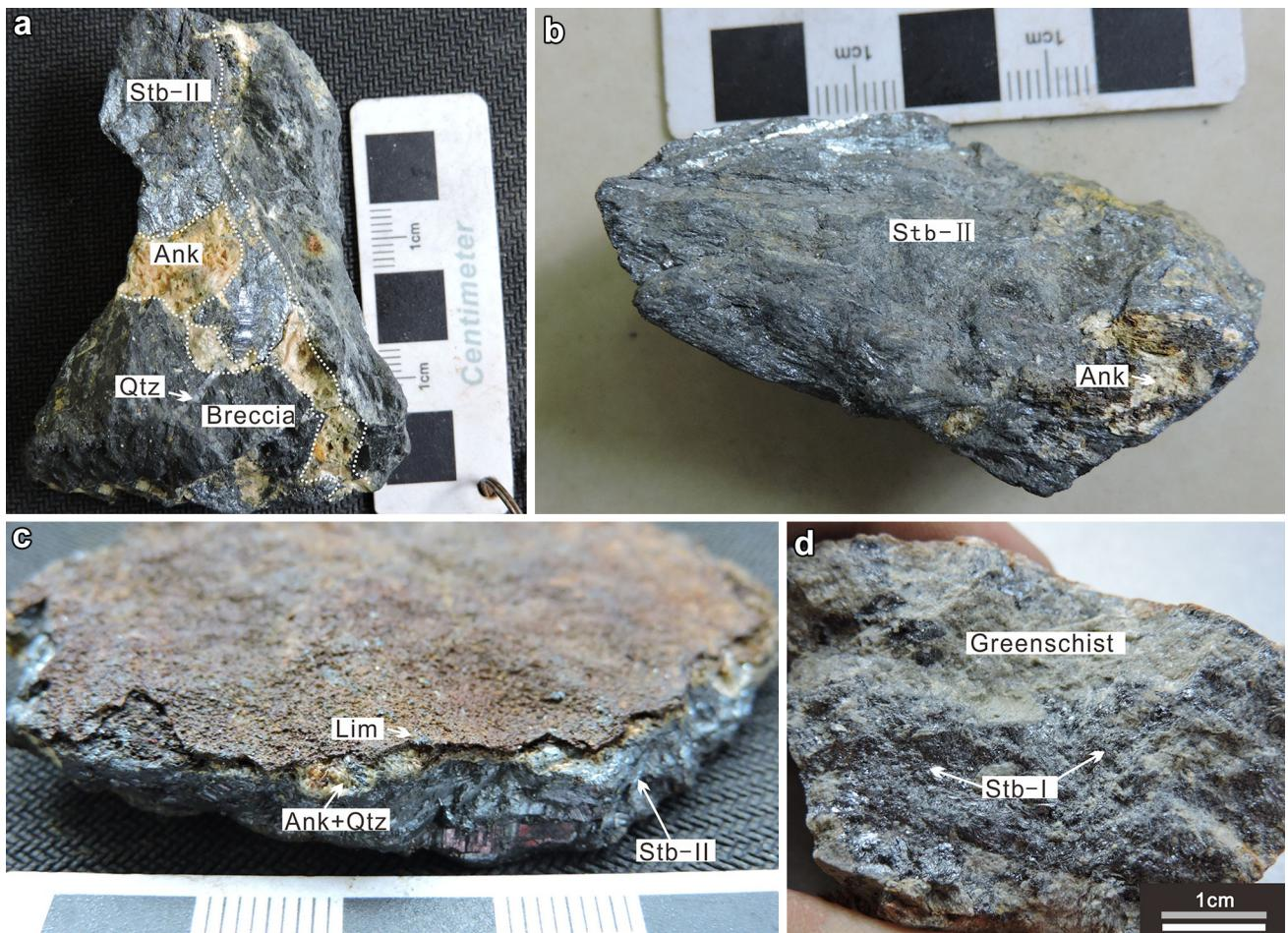
**Fig. 3** The main structures and tectonics of antimony ores of the Leishan-Rongjiang antimony ore field. **a** Breccia ore. **b** Drusy ore at the main-ore stage (Stb-II). **c** Bedded orebody in fault zone and altered minerals including ankerite, kaolinite, and limonite. **d** Disseminated ore of greenschist rocks at late-ore stage (Stb-I)
