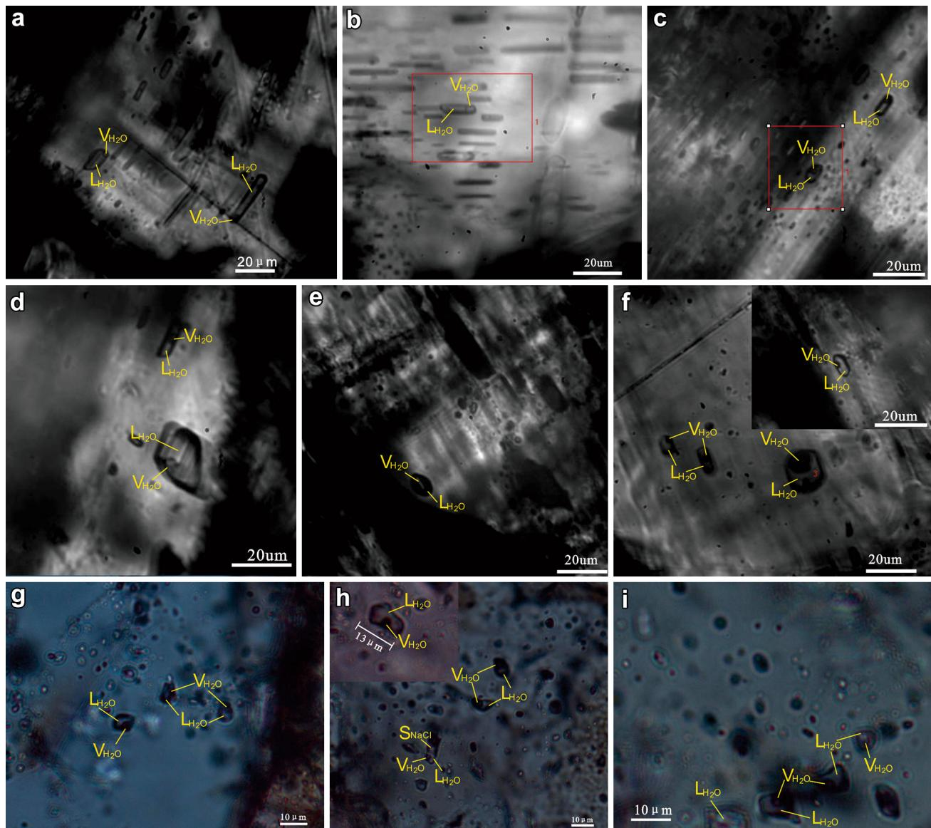
**Fig. 5** Photomicrographs of representative fluid inclusion types at room temperature in stibnite and coexisting quartz. **a–c** Type-I mass fluid inclusions in stibnite; **d–f** Type-IIa individual fluid inclusions in stibnite; **g–i** Type-IIb fluid inclusions in quartz
