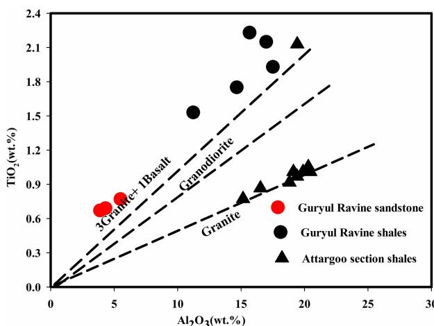
**Fig. 5**  $\text{Al}_2\text{O}_3$  versus  $\text{TiO}_2$  bivariate diagram (after McLennan et al. 1980)
