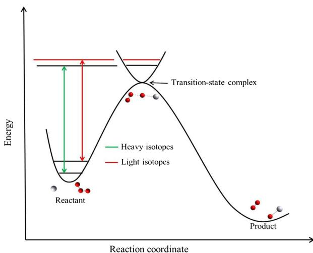
**Fig. 6** The classical transition state theory (TST) and the way it deals with a kinetic reaction. There is an activated complex at the highest potential energy place along the pathway from the reactant to the product (i.e., transition-state complex). The figure takes the kinetic reaction of Hg and O<sub>3</sub> as an example
