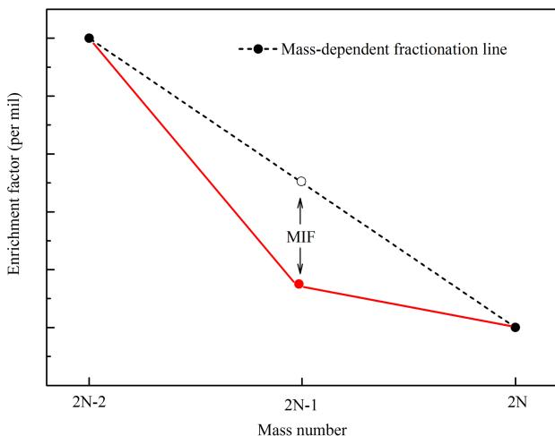
**Fig. 1** Variation of the enrichment factor with isotopes. N is a positive integer. The red line is the real fractionation line. The red solid circle (the odd number isotope) deviates from the mass-dependent line composed of even mass number isotopes
