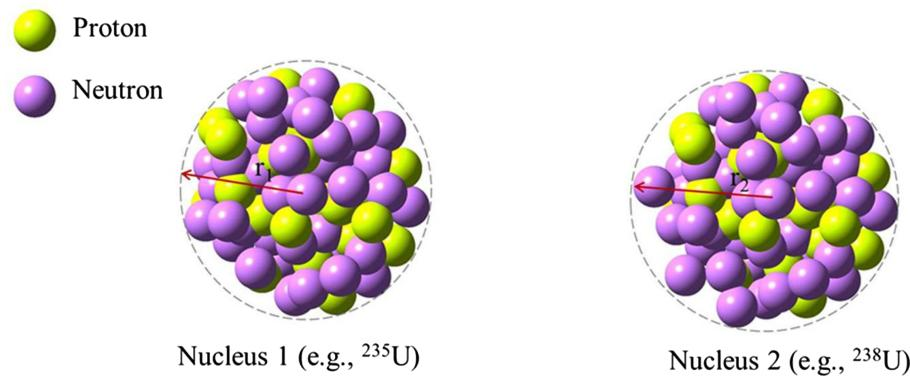
**Fig. 3** Nuclei of the isotopes of heavy elements with finite nuclear sizes. The different numbers of neutrons cause the difference in nuclear size and shape of isotopes (i.e., difference in nuclear radius  $r_1$  and  $r_2$ ). For example, the root mean-square nuclear charge radius  $\langle r^2 \rangle^{1/2}$  of  $^{235}\text{U}$  and  $^{238}\text{U}$  are 5.834 fm and 5.860 fm (Fricke and Heilig 2004), respectively
