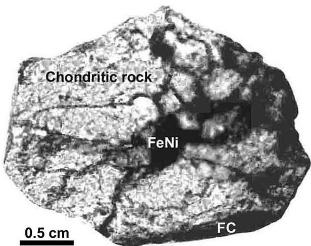
**Fig. 6** Photograph of a hand specimen of the Jilin meteorite showing an FeNi metal nodule connected with radiating and irregular fractures and net-shaped cracks. FC = fusion crust
