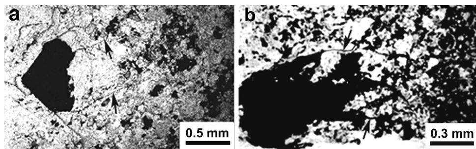
**Fig. 3** **a** A medium-sized metal grain No. 1 observed on the polished section prepared from the sample of Jilin No. 1 meteorite. Note the fine metal particles are remarkably decreasing around it and jointing with fractures of different directions. **b** A medium-sized metal grain No. 2 from sample G-62. Note its root-hair shape and jointing with fractures (parallel polarized light)
