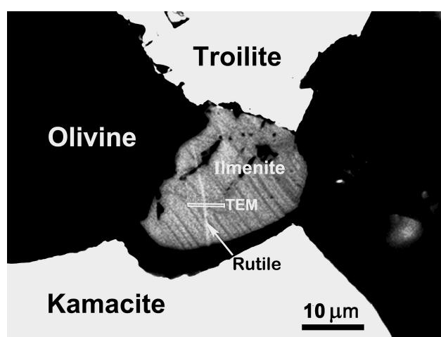
**Fig. 1** Acicular crystal of rutile in ilmenite surrounded by kamacite, troilite, and olivine, the line with TEM indicates the position of the TEM chip
