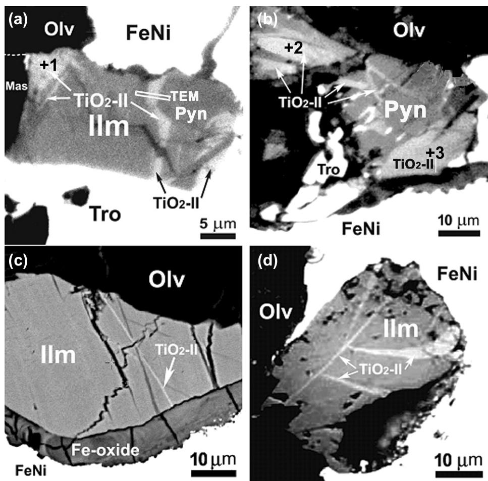
needle-shaped  $\text{TiO}_2\text{-II}$  of 40  $\mu\text{m}$  in length and 1.5–2  $\mu\text{m}$  in width. Interestingly, all  $\text{TiO}_2\text{-II}$ -bearing ilmenite grains we observed in the Suizhou meteorite are surrounded by FeNi metal or FeNi metal + troilite and olivine.
