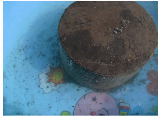
Fig. 8. Water immersion test of Chang 7 well core.
